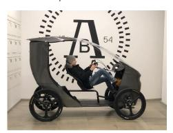
The vehicle is registered as a cargo ebike to be used in bike lanes and car free areas. It's required to peddle and has an ebike 250-500 W engine with max speed of 25km/h. The window and roof give substantial weather protection, and side doors can be added.
